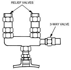
NOTE: The relief valve tree is available on all condensers. It is also applicable to Frame 4 machines with accessory isolation packages.
